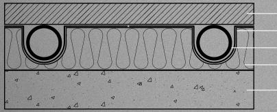
Engineered timber board Aluminium diffusion plate Oxygen barrier pipe Grooved EPS insulation
