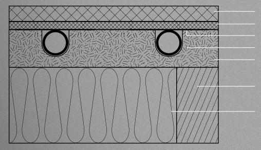
Finished floor 6mm engineered timber board Foil faced tape Oxygen barrier pipe Tongue & groove panel
