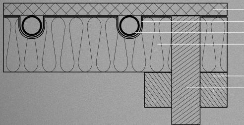
Finished floor Alumium diffusion plate Oxygen barrier pipe 50mm pre-grooved EPS insulation
