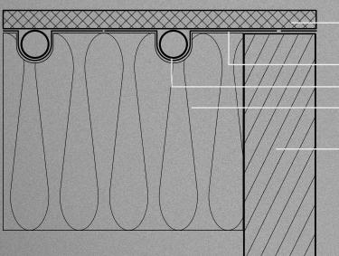
Aluminium diffusion plate Oxygen barrier pipe Quilted insulation
